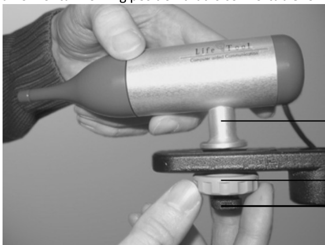
Illustration 2: Mounting the INTEGRAMOUSE® on the stand (housing base / lock nut / mounting screw)
