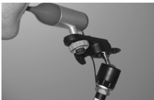
Illustration 5: INCORRECT — tilted positioning
