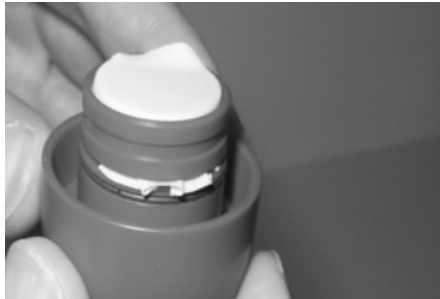
Illustration 11: INCORRECT — membrane fitted incorrectly
