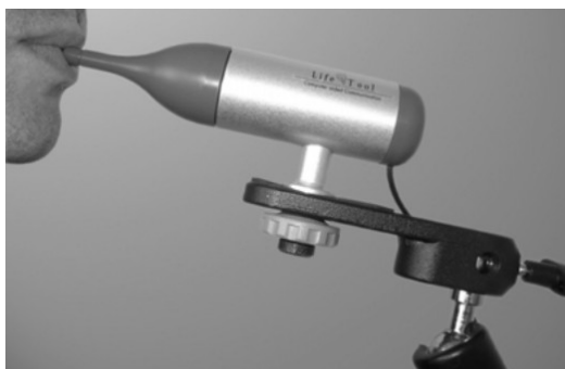
Illustration 4: CORRECT — horizontal positioning
