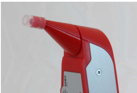
Figure 8: Correct placing of the silicon tube.
