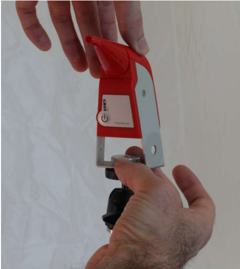
Figure 7: Installing the IntegraMouse Plus
