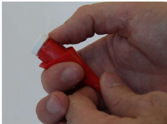
Figure 11: Removing the membrane
