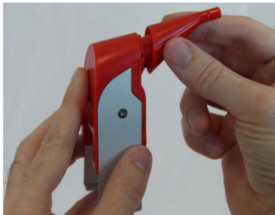
Figure 14: Placing the mouthpiece
