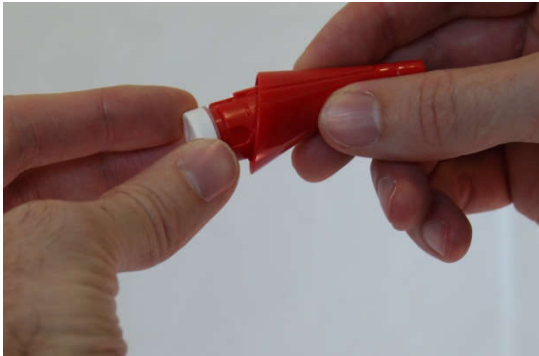
Figure 12: Placing the membrane
