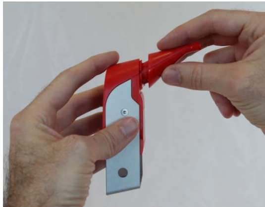
Figure 10: Removing the mouthpiece
